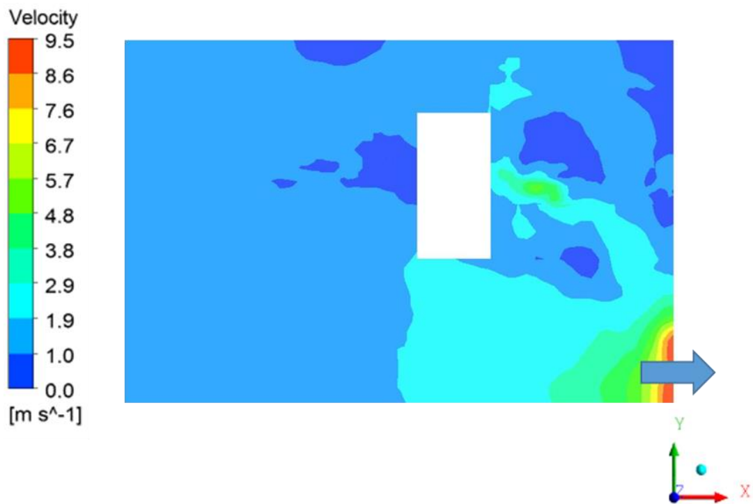
Figure 17 FDS velocity distribution at middle of height
